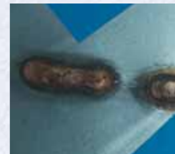
Galvanised steel sheet, MIG-brazed
